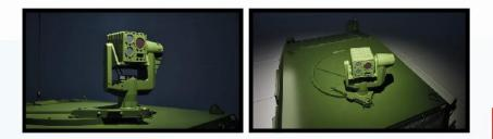
SEOM connects to remote weapon systems for enhanced targeting and features an operator console with a monitor-computer and joystick control for full system control.
